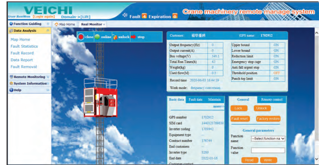
real time monitoring—Online monitoring of equipment operation, get related fault information.
