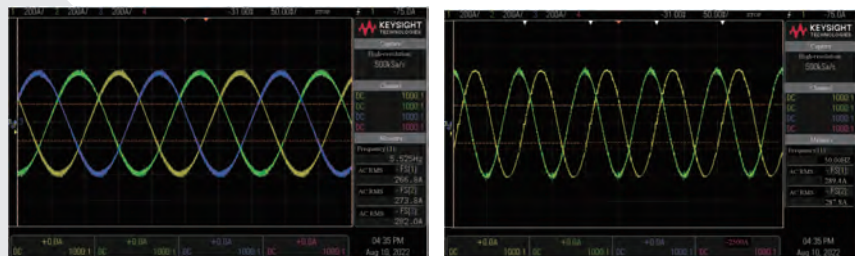
Harmonics to the motor <2% at rated load
