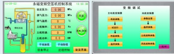
Air compressor special control system has high system integration, debugging on the touch screen and no need to set parameters on the inverter, it is simple to debugging.
