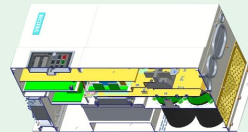
Strong adaptability to site environment, independent air duct, electrical components are not easily damaged by external corrosion, equipped with 24V high-speed dust-proof fan, can adapt to the harsh environment of the site and the high temperature.
