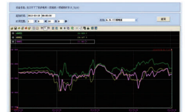
Daily Voltage Fluctuation Curve
