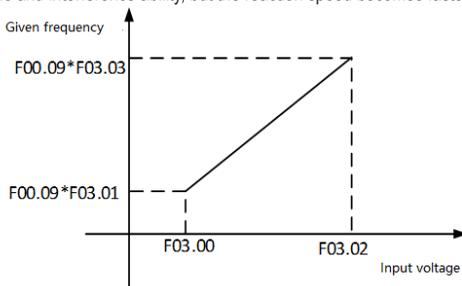
**Tips:** Set the frequency source to select AI1 timing, the set frequency can be adjusted to a negative value, and the [F00.16] hundred-bit selection frequency control direction can be matched to perform bipolar adjustment.
