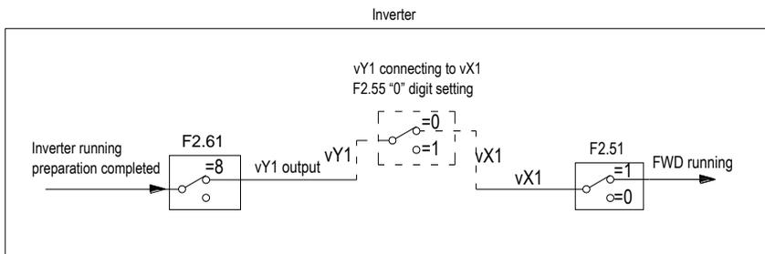
**Example 2: After the inverter is powered on, the delay is 60s forward running, as follows:**
