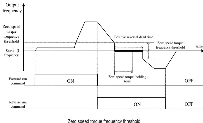
**Note:** If the zero speed holding torque is set too large or the zero speed holding torque time is set too long, pay attention to the temperature rise of the motor. If the motor temperature rises a lot, it is necessary to improve the heat dissipation of the motor plus the heat sink of the motor.
