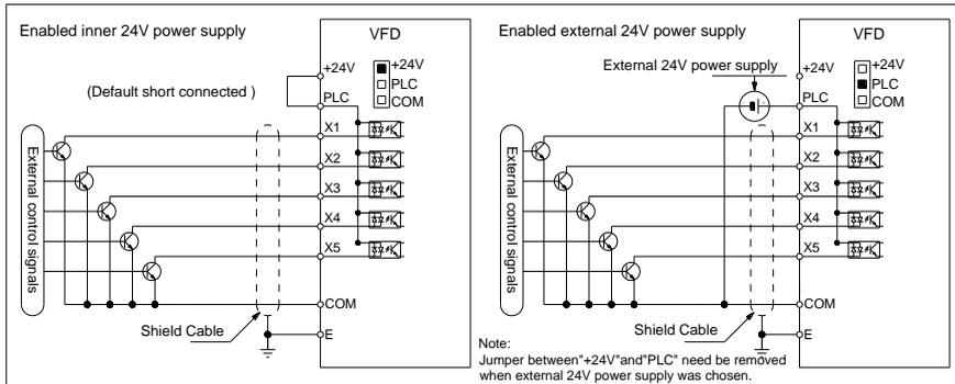
Jumper cap "+24V", "PLC", "COM" connection diagram:
