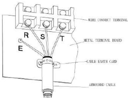
Chart 3-5: Cable earth card for cables grounding
