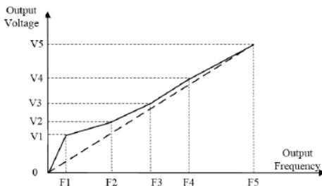
User sets the 1<sup>st</sup>/2<sup>nd</sup>/3<sup>rd</sup>/4<sup>th</sup>/5<sup>th</sup> voltage ratio of V/F curve corresponding to F1/F2/F3/F4/F5 frequency based on rated output voltage 100%. User sets the 1<sup>st</sup>/2<sup>nd</sup>/3<sup>rd</sup>/4<sup>th</sup>/5<sup>th</sup> frequency of V/F curve corresponding to V1/V2/V3/V4/V5.
