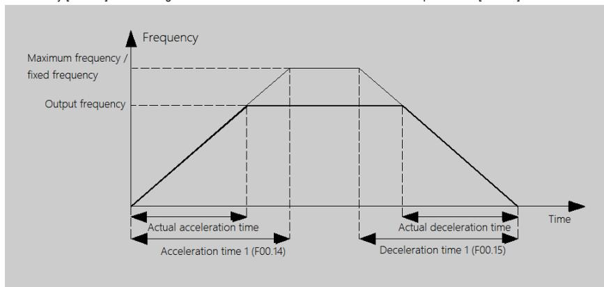
Four groups of acceleration and deceleration time can be selected for normal frequency acceleration and deceleration. Acceleration / deceleration time 1 is set by [F00.14~F00.15], acceleration/deceleration time 2, acceleration
