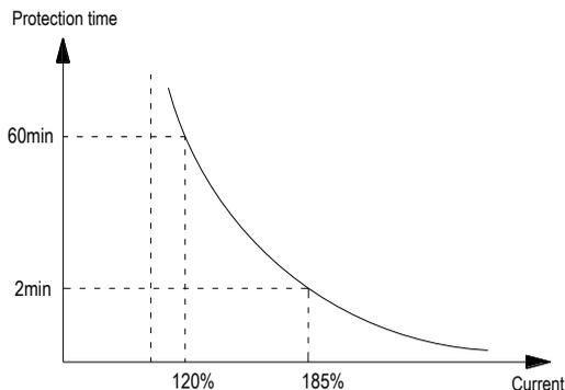
The current entering protection curve= (the real motor current / oL protection coefficient) $\times$ 110%
