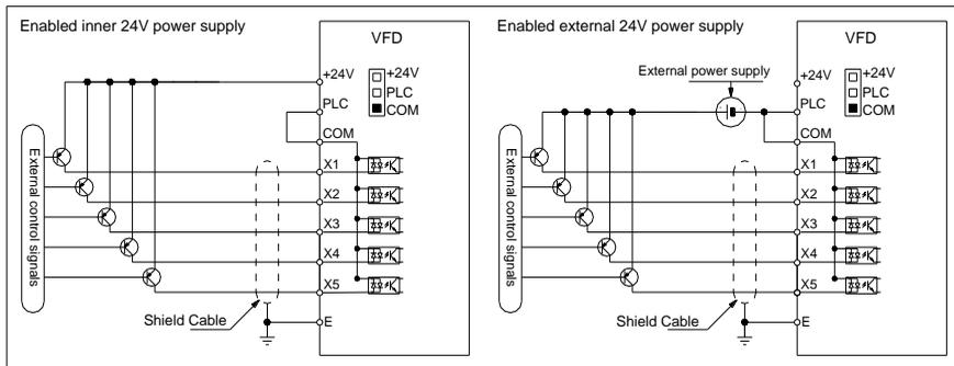
NPN transistor connection mode:
