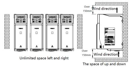
Figure 3-3: Installation space requirements
