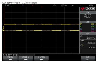
Measure the voltage of each drive signal and GND is about 11.5v when running with ACgear.
