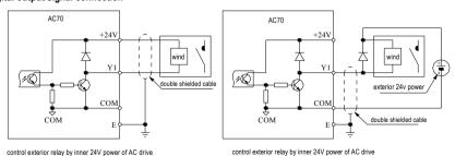
Chart 3-26:AC70 series AC drive digital output signal connection mode
