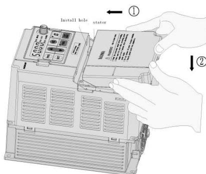
**Dismantlement:** At the tail of the AC drive, there is a special dismantlement hole design. Put your finger into the hole, upwardly pull the cover with a little force until the buckle between the tail-hood and the crust tear off, and then remove the tail-hood down.
