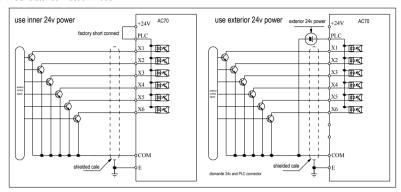
Chart 3-24: NPN transistor digital input signal connection mode
