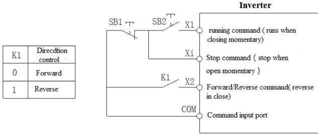
**Tip:** In 3 wire control mode 1 Fig, SB1 is a normal close stop button, SB2 is a normal open button. K1 is a direction selection switch; Xi is multi-function terminal (X1-X6) which have been programmed for 3 wire running control terminal.
