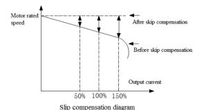
If cooperate with auto torque boost function, the torque performance in low frequency characteristic of AC drive will be significantly improved. The value of slip frequency compensation should be set base on motor rated slip, should not set the value of compensation too large.
