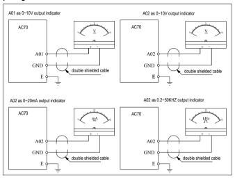
Chart 3-27:AC70 series AC drive analog output signal connection mode Connection of pulse input signal
