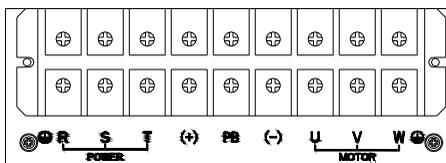
Arrangement sequence of main circuit terminal with 37~110kW
