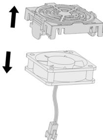
3, Poke the clips toward the outside and detach the fan from the cover by a little strength.
