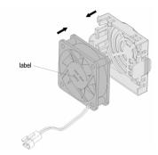
1, Install the fan vertically into the cover as shown in the picture (the label should face the outside).
