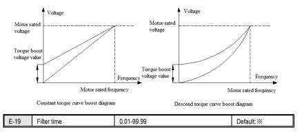
This function mainly used to torque boost in OLV control mode. The value setting is smaller, the response of torque boost is faster, the fluctuation of current is bigger, suitable for sudden changing load application; vice versa, the filter time setting is bigger, the response of torque boost is slower, the fluctuation of current is smaller, suitable for constant load application.
