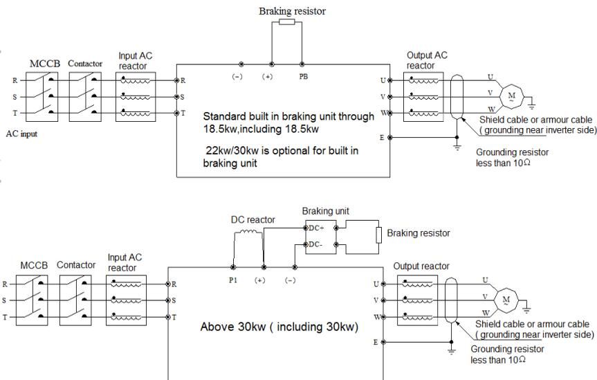
Chart 3-19: AC70 AC drive main circuit wiring
