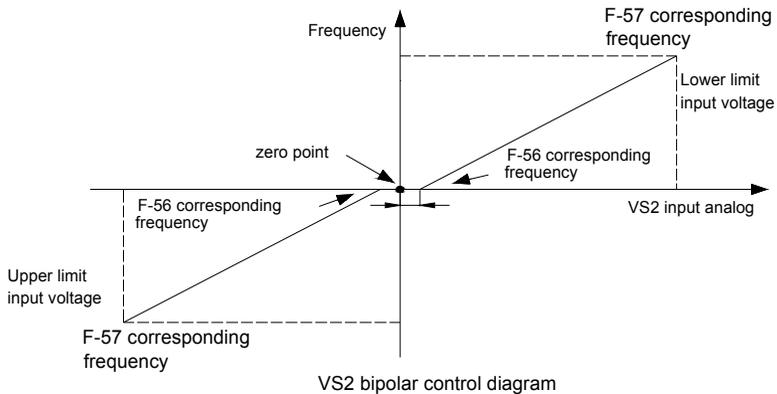
**Tip:** When (VS2) is used as PID given or feedback channel, the function of bipolar is invalid. At this moment, the usage of (VS2) terminal is the same with the (VS1) terminal. Namely, when (VS2) <0, AC drive think the input of this port is 0.
