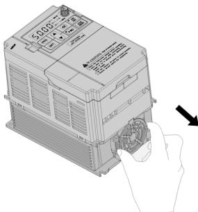
1, Pinch the two elastic clips of the fan and pull out. Then dismantle the fan cover.
