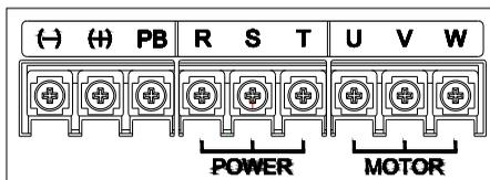
Arrangement sequence of main circuit terminal with 22~30KW (standard machine without PB terminal) (22KW for steel cover machine)
