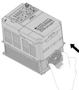
3, Insert the two elastic clips of the fan cover vertically into the fan installation slots.
