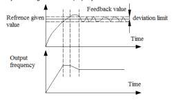
PID control deviation limit diagram
