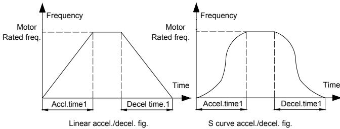
**LED tens digit: Accelerate/decelerate time datum point.**
