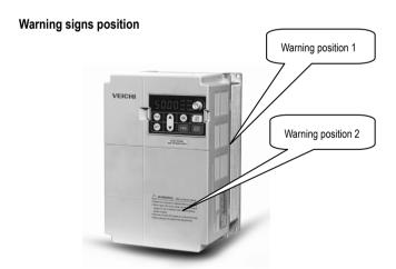
Drawing 1: Warning positions on crust of AC70 series AC drive
