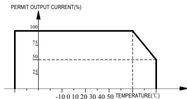
**Chart 3-2: AC70 series AC drive derating curve while over permit temperature**
