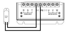
Fig 3-22: AC70 Series AC drive Brake resistance wiring of machine with 22KW and 30KW(built-in brake is optional) (22KW for steel cover machine)
