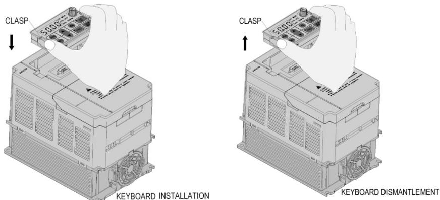
Chart 3-17: AC70 series AC drive keyboard installation and dismantlement
