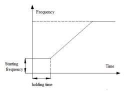
Starting frequency and holding time schematic
