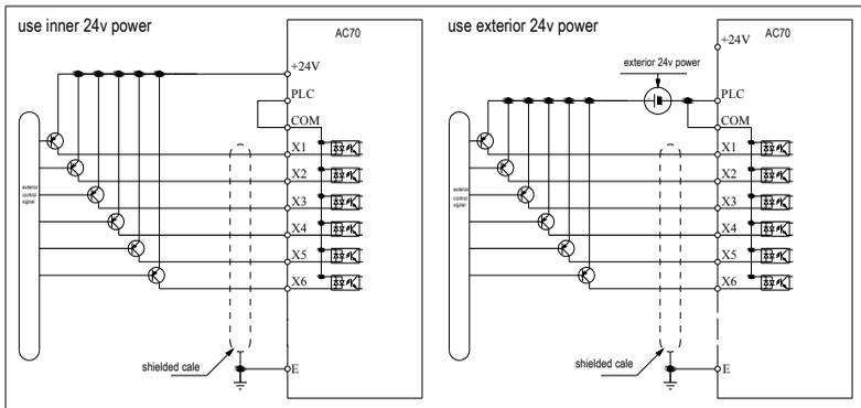
**Chart 3-25 PNP transistor digital input signal connection mode**
