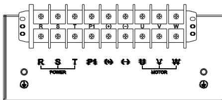
Arrangement sequence of main circuit terminal with 132kW:
