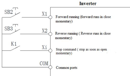
**Tip:** 1. SB2 and SB3 both are normal open button, and enable by pulse edge.
