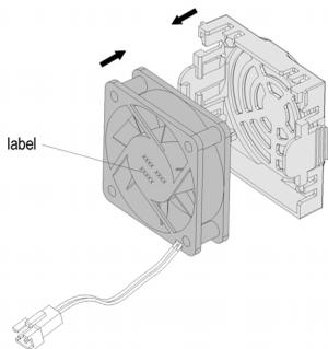
1, Install the fan vertically into the cover as shown in the picture (the label should face the outside).
