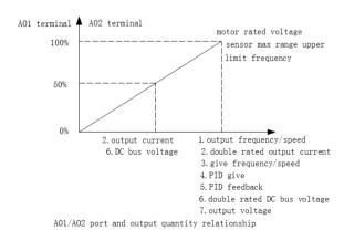
Tips: when (AO2) port is frequency pulse output or 4-20mA output, '0%' corresponding output quantity is not zero.
