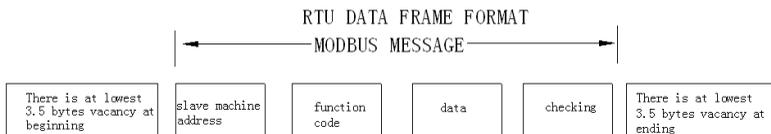
One frame message must be transmitted as a continued data flow. If there is a pause over 1.5 byte before the end, the receiving equipment will clear the half-baked information. And the next byte will be considered as the address domain of
