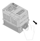
1, Pinch the two elastic clips of the fan and pull out. Then dismantle the fan cover.
