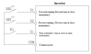
Tip: 1. SB2 and SB3 both are normal open button, and enable by pulse edge.
