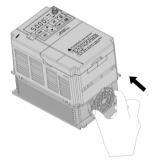
3, Insert the two elastic clips of the fan cover vertically into the fan installation slots.
