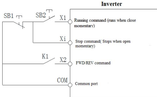
**Tip: SB1 is a normal stop button, SB2 is a normal open button. K1 used for running direction selection button. Xi is multi-function terminal (X1-X6) which have been programmed for 3 wire running control terminal.**
