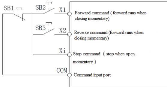
**Tip:** In 3 wire control mode 2 Fig, SB1 is a normal close button, SB2 and SB3 both are normal open button and pulse edge is valid, uses for AC drive direction control.
