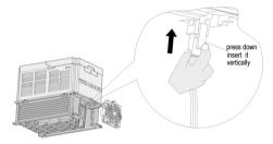
2, Press the elastic clip of the fan by finger toward the inner side and insert the leading terminal of the fan vertically by a little strength.
