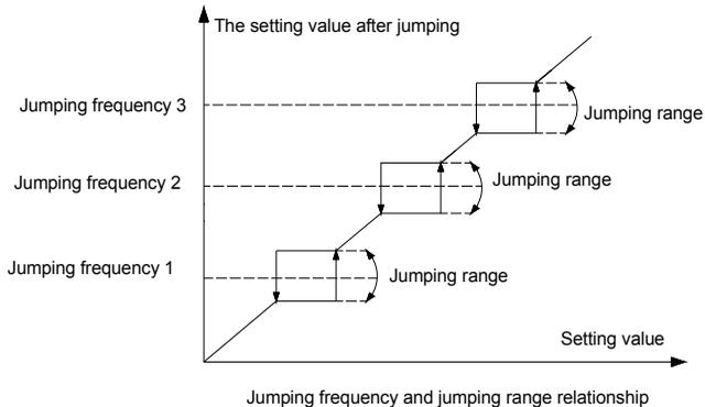
**Note: 1. The output frequency still will pass the jumping range during acceleration or deceleration. Make sure the parameters don't overlap or inset setting.**
