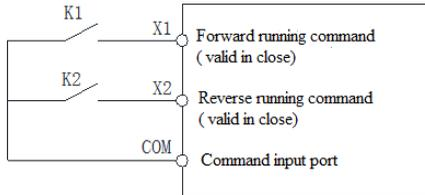
**1: Two wire running control mode** Running and direction are separated. Uses the forward running terminal X1 (forward running) to determine running control, reverse running terminal X2 (reverse running) to determine direction control. Refer to below fig.
