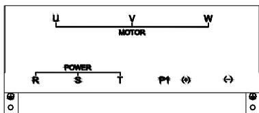
Arrangement sequence of main circuit terminal with 160~560kW
