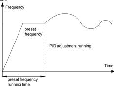
PID preset frequency running time diagram
