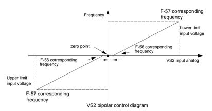
Tip: When (VS2) is used as PID given or feedback channel, the function of bipolar is invalid. At this moment, the usage of (VS2) terminal is the same with the (VS1) terminal. Namely, when (VS2) <0, AC drive think the input of this port is 0.
