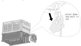
2, Press the elastic clip of the fan by finger toward the inner side and pull out the leading terminal of the fan vertically by a little strength.
