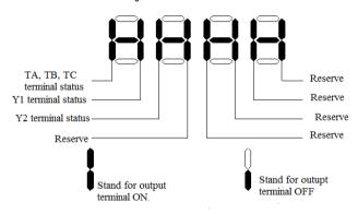
Output terminal ON/OFF status diagram
