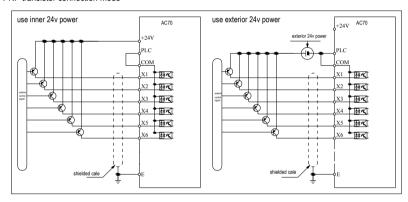
Chart 3-25 PNP transistor digital input signal connection mode
