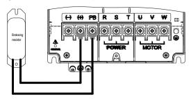
Fig 3-21: AC70 Series AC drive Brake resistance wiring of machine with 15-22KW (for plastic cover machine)
