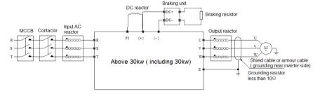
Chart 3-19: AC70 AC drive main circuit wiring
