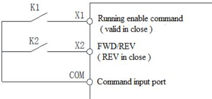
**2. Three wire control mode 1** Three wire control terminal (Xi) is used for stop running terminal. Running command determined by forward running terminal X1 (forward running), direction determined by reverse running terminal X2 ( reverse running). 3 wire running control terminal Xi is used for enable input.
