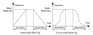
LED tens digit: Accelerate/decelerate time datum point.
