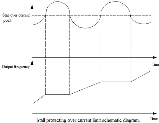
This parameters datum line is rated current of AC drive. It will extend acceleration time longer. It means the current limit function is activated if the frequency can't accelerate to set value or frequency given, but fluctuates in the fixed frequency range. Please reduce the load or adjust the some relevant parameters.
