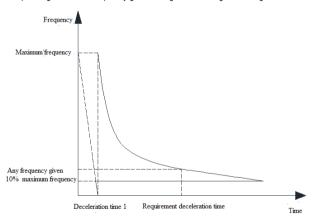
Equidistance deceleration time schematic diagram
