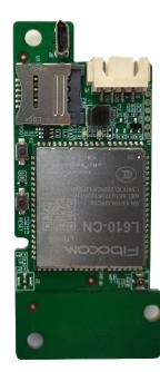
IOT-BMC410 is an IoT wireless data terminal 4G product that uses public cellular network to provide users with wireless long-range secure and reliable data transmission function.
