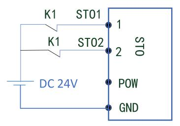
Diagram of wiring of internal power supply:
