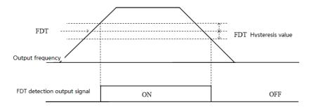
Frequency level detection diagram
