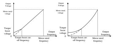
Torque lifting diagram
