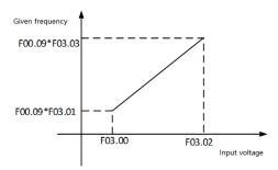
Tips: Set the frequency source to select AI1 timing, the set frequency can be adjusted to a negative value, and
