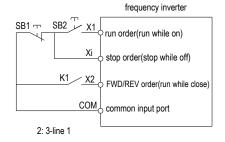
2: Three-wire control 1 schematic
