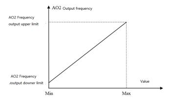
AO2 port pulse frequency output diagram
