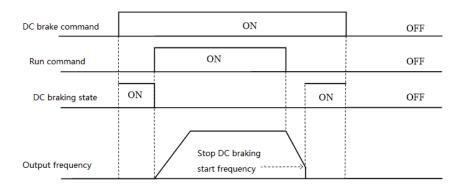
DC braking command diagram
