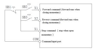
3: Three-wire control 2 schematic
