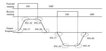
Schematic diagram of S curve
