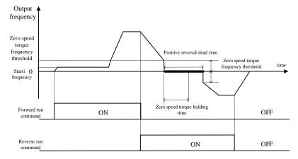
Zero speed torque frequency threshold
