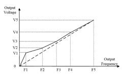
User sets the 1st/2nd/3rd/4th/5th voltage ratio of V/F curve corresponding to F1/F2/F3/F4/F5 frequency based on rated output voltage 100%. User sets the 1st/2nd/3rd/4th/5th frequency of V/F curve corresponding to V1/V2/V3/V4/V5.
