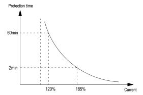
The current entering protection curve= (the real motor current / oL protection coefficient)x110%
