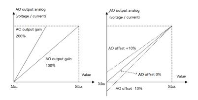
AO analog output and gain, offset schematic
