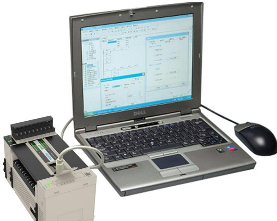
Figure 1-5 Programming cable connection
