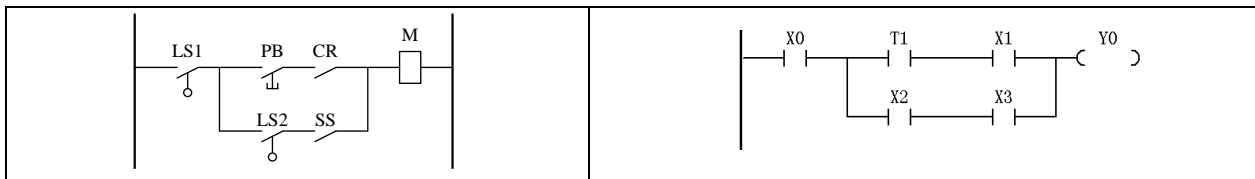
Figure 4-1 The equivalence between electrical control diagram and LAD
