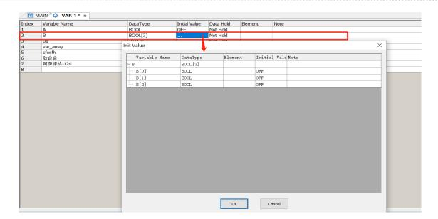
When an array is used in the command, the access starts from the element specified by the subscript of the array.
