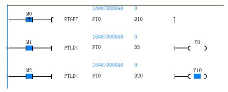
The PT< instruction checks the address of the pointer type variable PT0 to determine whether it is greater than the D address, e.g., if the PT0 pointer points to D10, a comparison with D5 will output Y0 as OFF, and a comparison with D20 will output Y10 as ON. similar check instructions PT>=, PT<, PT<=, PT=, PT<> can implement the PT pointer pointing judgment check
