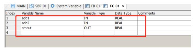
In the Input-Output and Local Variable Definition window, you can define input (IN), output (OUT), input-output (INTOUT) and local variables (VAR) for function blocks. Variable data types support BOOL, INT, DINT and REAL, and array variables and structures can be defined. If a structure variable is used, the Structure members need to be created in the structures of global variables.
