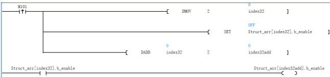
After M101 is triggered, Struct\_arr[2].b\_enable is set, and according to its state, Struct\_arr[3].b\_enable is controlled:
