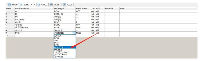
Pointer type variables can do address operations and indirect addressing operations. When using the pointer address operation instruction, it indicates the address operation of a pointer. The instructions that support pointer address operations are listed below. When using these instructions, the functions of fetching address, pointer address offset, and pointer address comparison are implemented.
