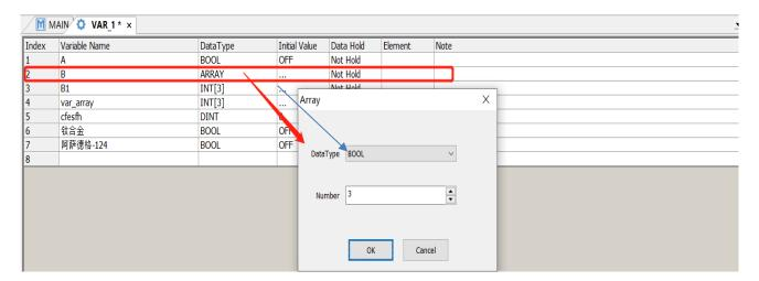
2. Click the initial value column of the array variable to enter the initial value setting interface of the array variable:
