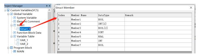
After creating structure and member variables, you can define structure variables by selecting structure in the data type of variable definition
