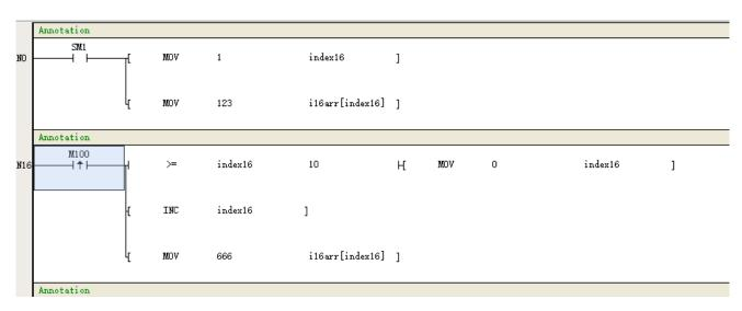
Start assigning 123 to i16arr[1], after that, each time M100 is triggered, it will assign 666 to the array elements behind it in a smooth manner; after starting:
