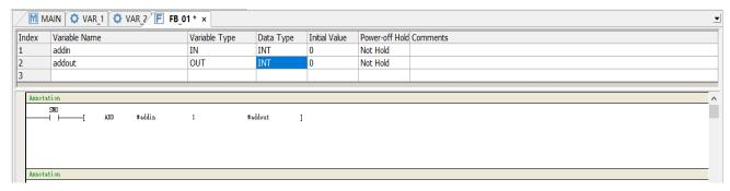
After M102 is triggered, the value 88 is assigned to i16arr [2], and after FB calculation, the value is assigned to i16arr
