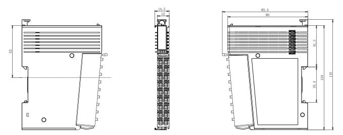
Ensure at least 10mm of clearance above the product to accommodate the latch's movement.
