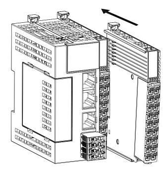
Description: Depress the rail latch to open it, then place the module on the DIN lead rail and press down on the latch to secure it. Install a DIN snap on both the master and modules. When installing the rail snap, hook the bottom of it to the bottom of the rail and then rotate the snap so that the top end of it is hooked to the top end of the rail, and finally tighten the screws to lock the rail snap.
