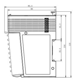
Ensure at least 10mm of clearance above the product to accommodate the latch's movement.
