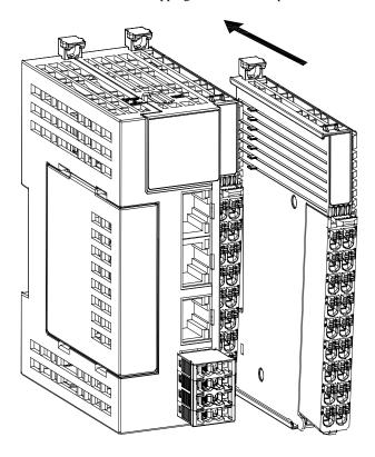
Description: Depress the rail latch to open it, then place the module on the DIN lead rail and press down on the latch to secure it. Install a DIN snap on both the master and modules. When installing the rail snap, hook the bottom of it to the bottom of the rail and then rotate the snap so that the top end of it is hooked to the top end of the rail, and finally tighten the screws to lock the rail snap.
