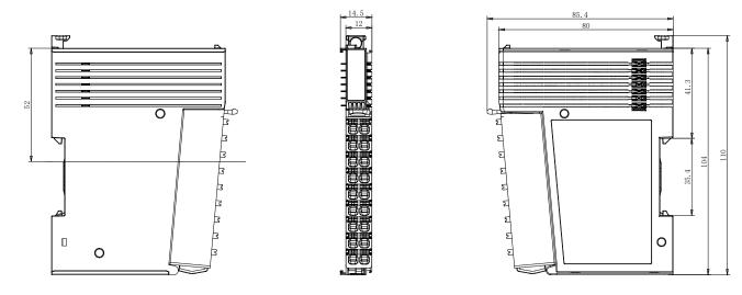
Ensure at least 10mm of clearance above the product to accommodate the latch's movement.
