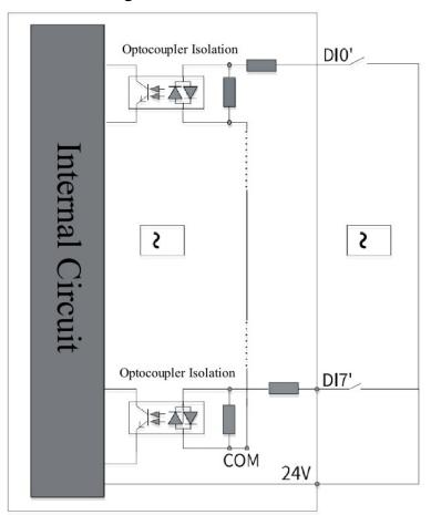
Note: The VH-0808ETP module is fixed with source type input configuration.
