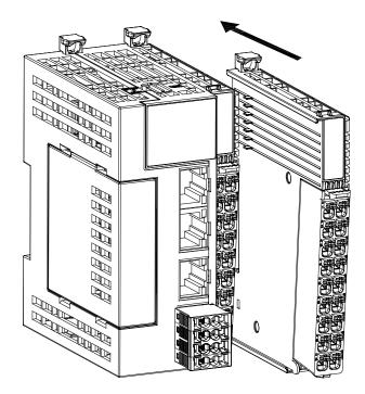
Description: Depress the rail latch to open it, then place the module on the DIN lead rail and press down on the latch to secure it. Install a DIN snap on both the master and modules. When installing the rail snap, hook the bottom of it to the bottom of the rail and then rotate the snap so that the top end of it is hooked to the top end of the rail, and finally tighten the screws to lock the rail snap.
