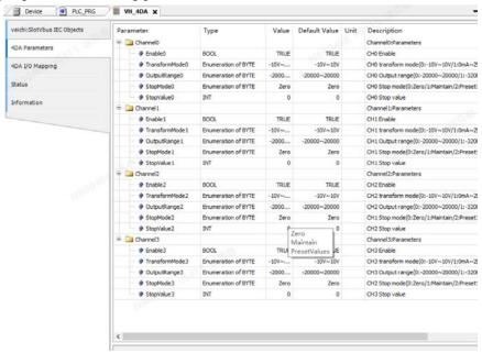
2. After logging on on-line, double-click the VH-4DA module to pop up 4DA parameter configuration, modify channels and switch modes as needed, and set sampling time and filtering parameters.
