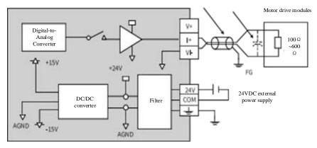
Note: \*1 Use two-core twisted shielded cables for analog signal lines.
