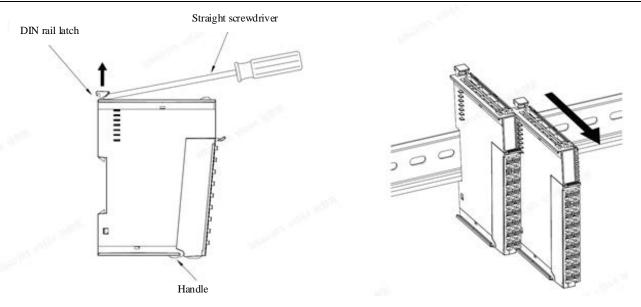
Depress the rail latch with your finger and then pull the module away from the DIN lead rail.
