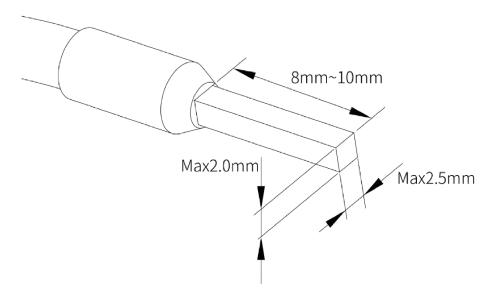
Electrical Installation VH-4DA Module Manual
