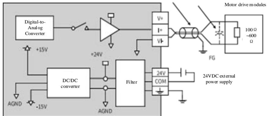
Note: \*1 Use two-core twisted shielded cables for analog signal lines.
