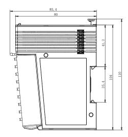
Ensure at least 10mm of clearance above the product to accommodate the latch's movement.
