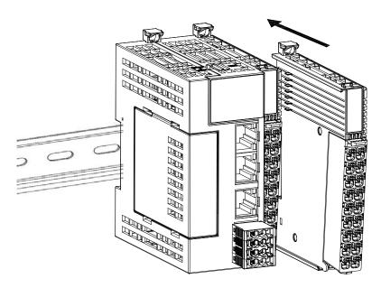
**Note:** Depress the rail latch to open it, then place the module on the DIN lead rail and press down on the latch to secure it. Install a DIN snap at both ends of the main unit or module. When installing the rail snap, hook the bottom of it to the bottom of the rail and then rotate the snap so that the top end of it is hooked to the top end of the rail, and finally tighten the screws to lock the rail snap.
