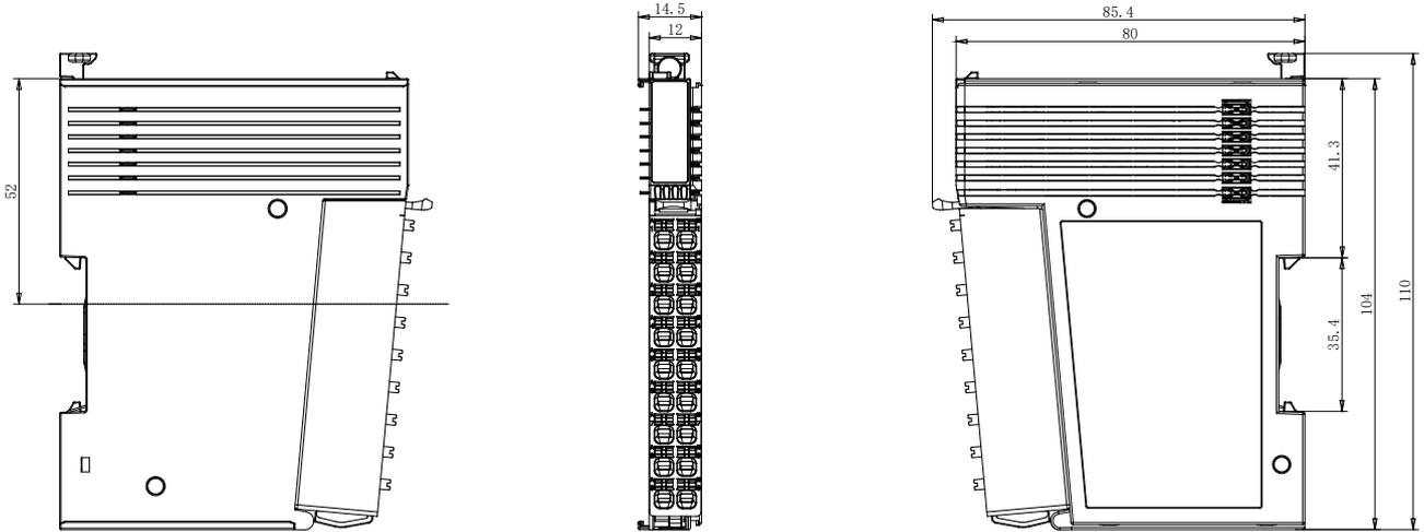
Ensure at least 10mm of clearance above the product to accommodate the latch's movement.
