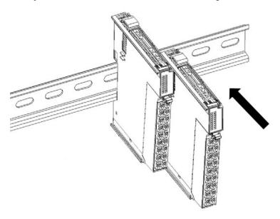
**Note:** Push the rail snaps first to open state, place the module onto the DIN rail, press down the top of the snaps with your hand until it is in place. Install a DIN rail clamp at each end of the main unit or module and when install them, hook the bottom of the DIN rail clamp to the bottom of the DIN rail and
