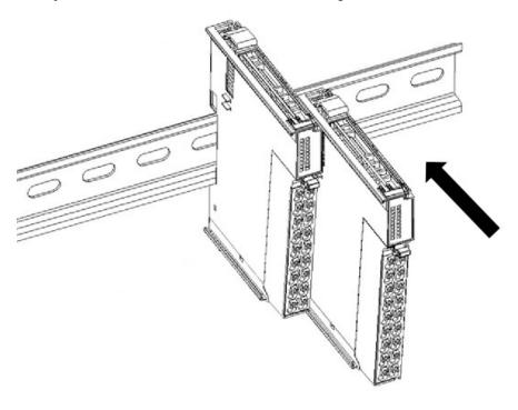
**Note:** Push the rail snaps first to open state, place the module onto the DIN rail, press down the top of the snaps with your hand until it is in place. Install a DIN rail clamp at each end of the main unit or module and when install them, hook the bottom of the DIN rail clamp to the bottom of the DIN rail and then rotate the DIN rail clamp so that the top end of the DIN rail clamp is hooked to the top end of the DIN rail, and then finally tighten the screws to lock the DIN rail clamp.
