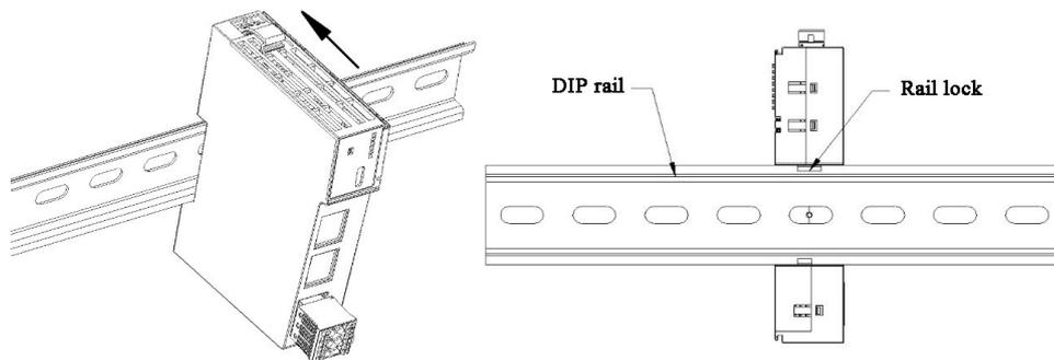
**Note:** After the module installation is completed, the snap will automatically rebound to lock the DIN rail, if the snap does not rebound, please press it down on the top of the snap by hand to ensure that the installation is in place.
