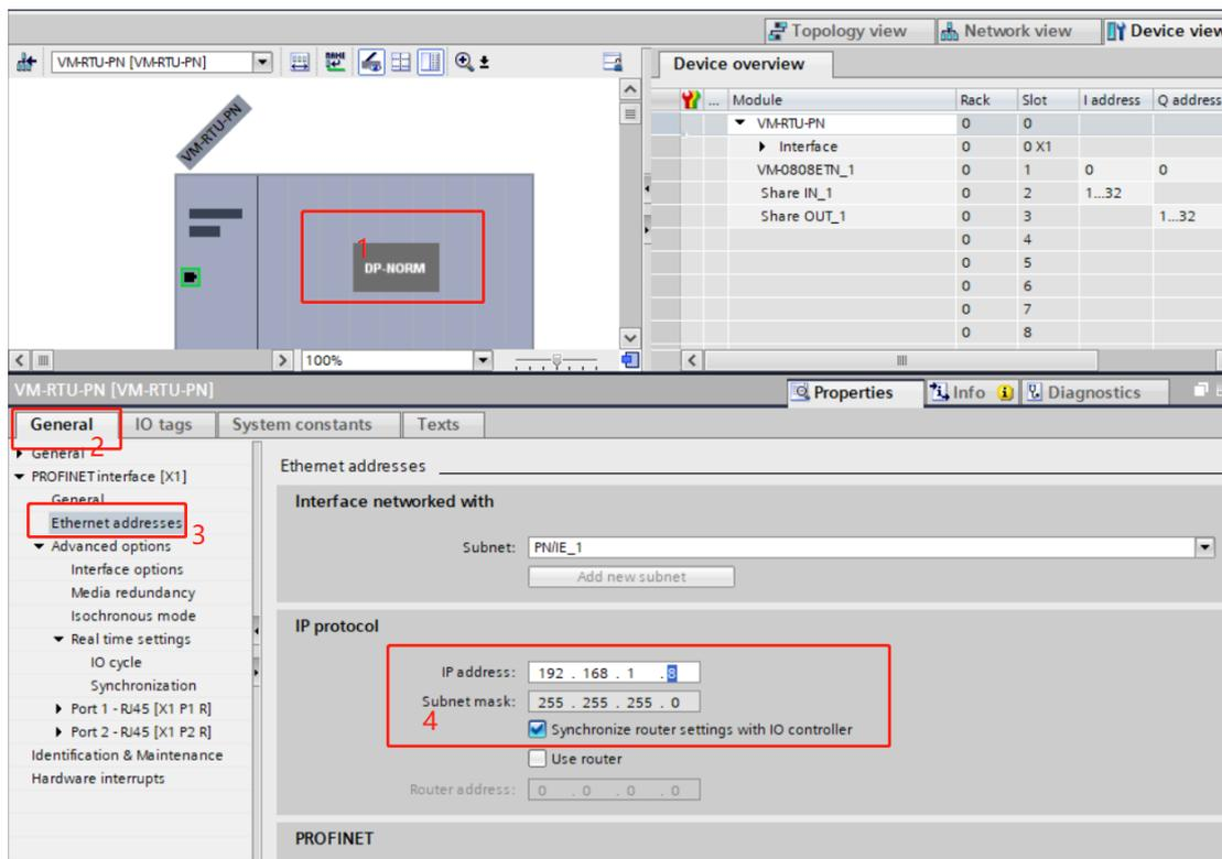
Figure 7 Slave IP address setting
