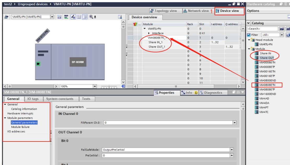
Figure 5 Module configuration
