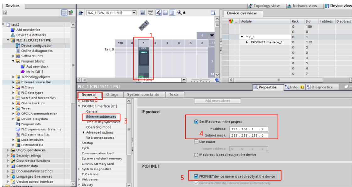
Figure 6 Master IP address setting
